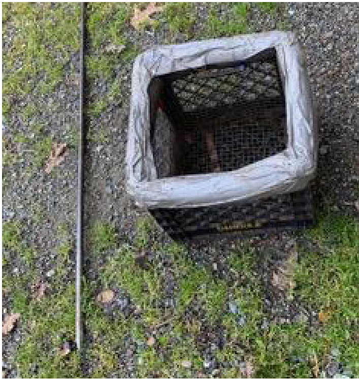
Soil Digger next to One Person Sieve. Note that the sharp edges are covered with pool noodles or pipe insulators and covered with tape and wire.
